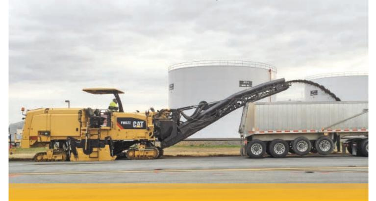
The PM622 is a highly productive, highly maneuverable half-lane milling machine that performs controlled full-depth removal of asphalt and concrete pavements in a single pass.
