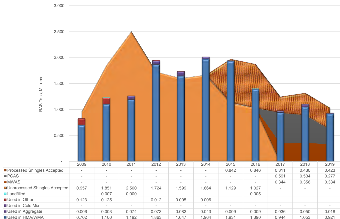
Figure 9: Comparison of Tons of RAS Accepted and Tons of RAS Used or Landfilled (Million Tons), 2009–2019. Processed RAS Acceptance First Tracked in 2015
