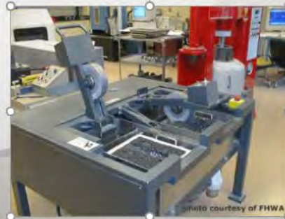
Lab Test (Hamburg Wheel Tracker)
