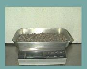
Dry the sample to constant mass @ 110 ± 5° C (230 ± 9° F) and determine the mass of the test sample.
