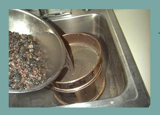
Immediately pour the wash water over the nested sieves avoiding the decantation of coarser particles of the sample.
