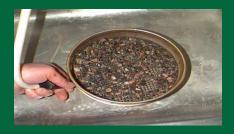
· Care should be taken to not cause abrasion to the sample during washing · Dry fraction to constant weight at 110  $\pm$  5 ° C
