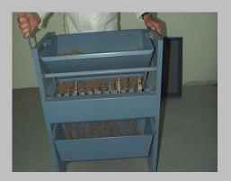
Splitting continued from one side until sample reduced to required specimen size
